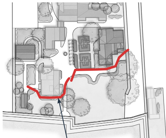
Proposed locations of Emergency Deployable Barrier
